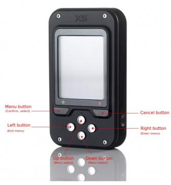
Figure 4: The Buttons on the X5
