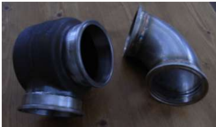
Outlet after fitting replacement flanges and an alternative solution using a 90° stainless bend
