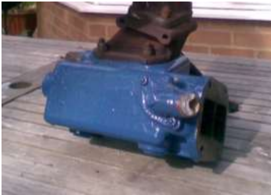
Cast aluminium exhaust manifold extension (blue) with turbo mounting.
