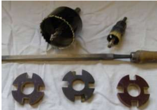
Drive disc in the centre clearly showing wear due to age and vibration
