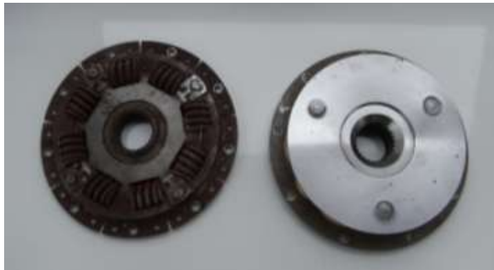
Original drive plate and modern replacement
