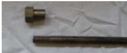
Machined blind nut which holds the header tank together
