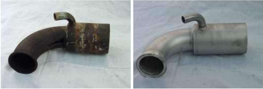
Original Perkins exhaust outlet showing heavy corrosion and a replacement exhaust manufactured from 316 stainless
