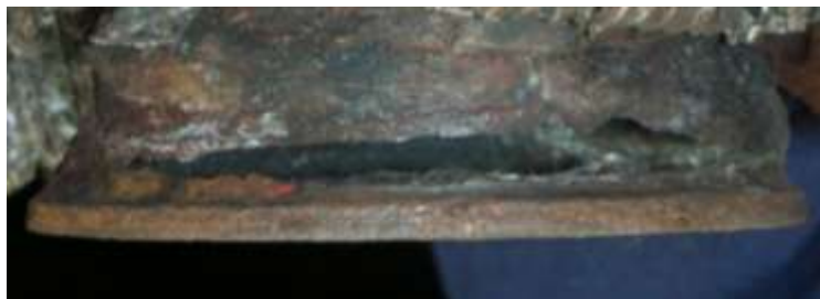
Corroded flange with large hole
