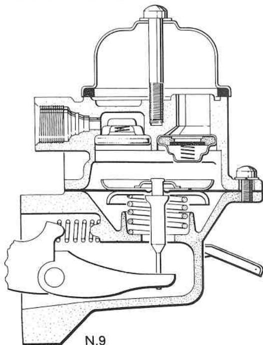
The valves are "staked in" and can be prised out using a screwdriver or other suitable tool. Clean the casting so that new valves can be correctly seated.
