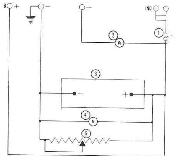
Test Circuit for 17ACR alternators. Standard terminations, battery-sensed.
