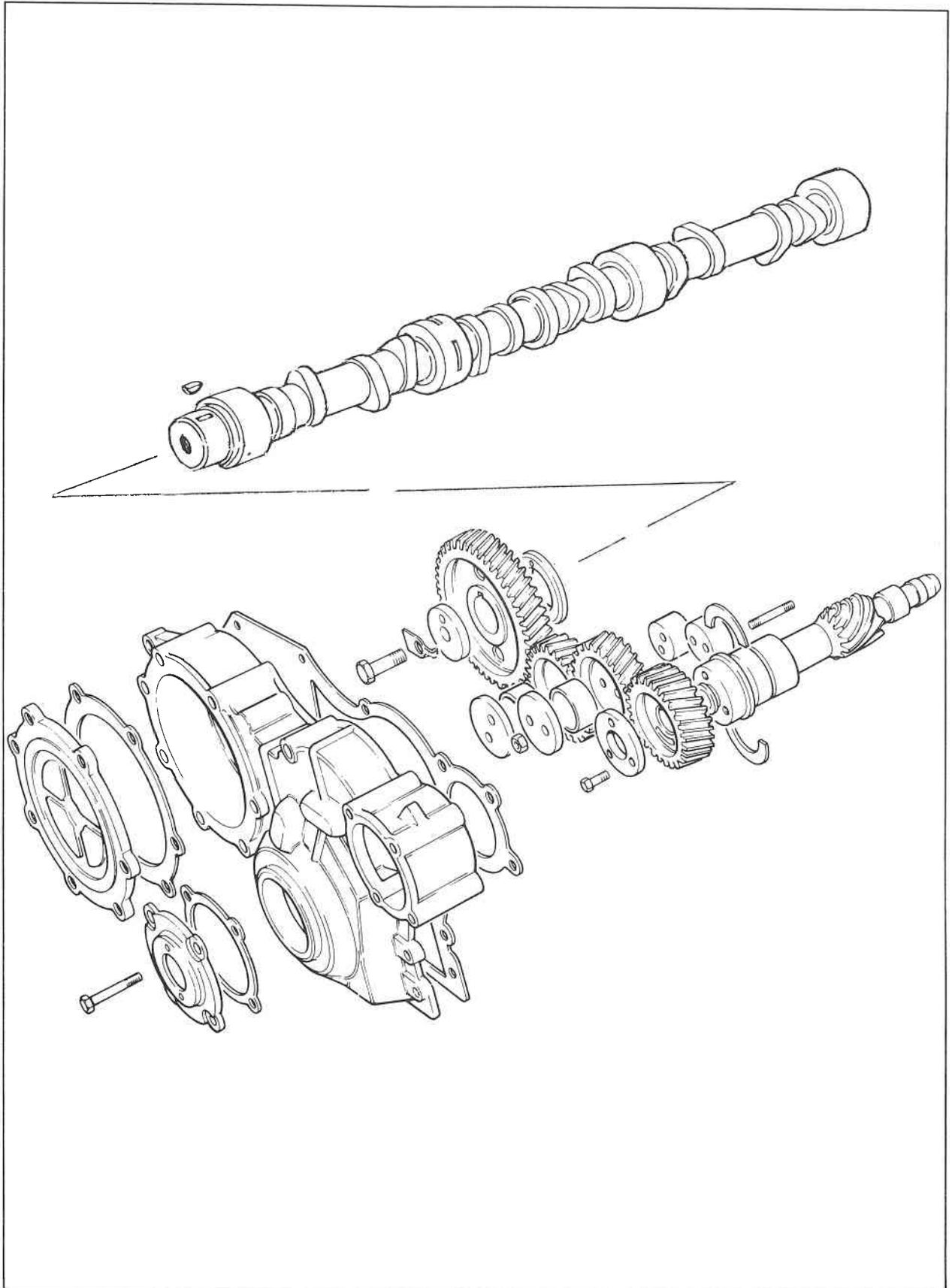
**To Remove Timing Case, Camshaft Gear and Auxiliary Drive Gear**
