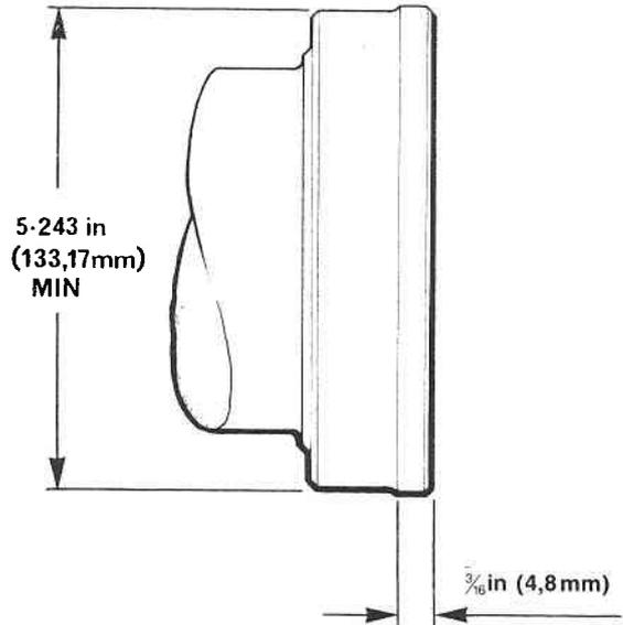
Using clean engine lubricating oil, lubricate the outside diameter of the seal and the inside diameter of the housing.
