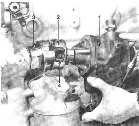
Fig. T.2. Removing Exhauster.
