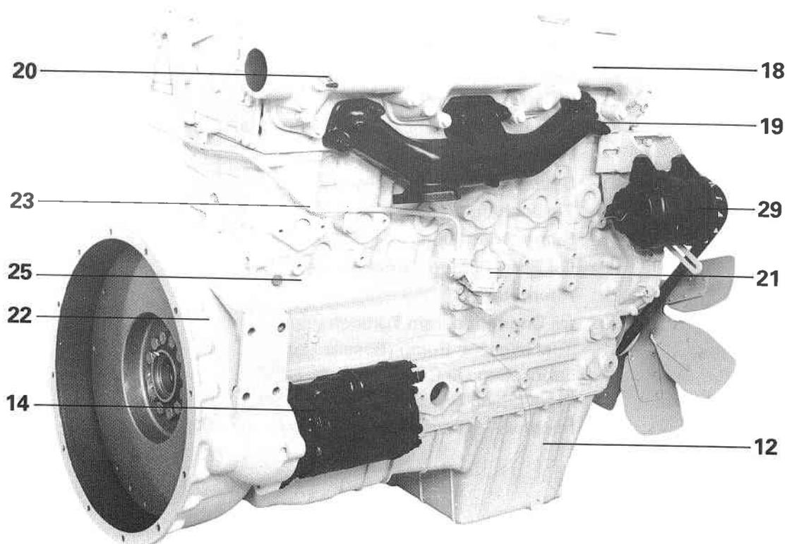
A.2 View of Camshaft Side of 6.3544 Engine
